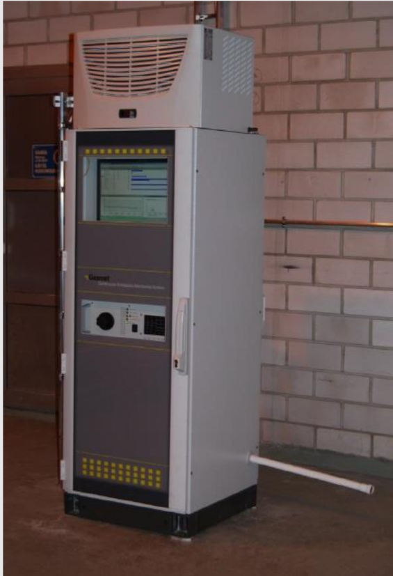
Abb. FTIR Monitoring System (links). Belebung der KA Helsinki in 20 m Tiefe. Fotos: Sanna Alku, HSY, Gasmet CX4000 FTIR
